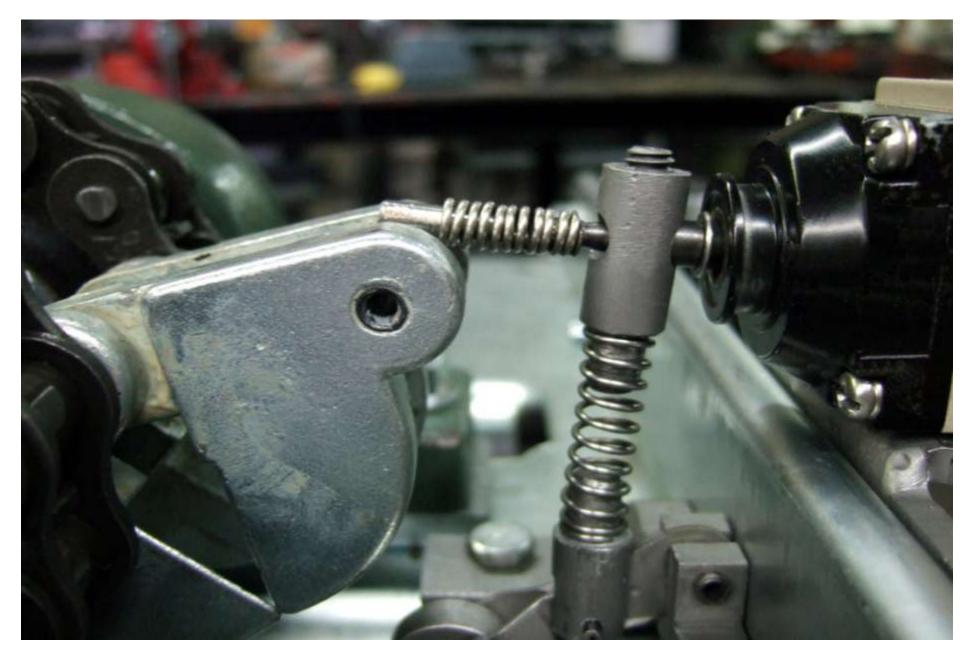
**Bridgeveyor D-2000 Jam Prevention Switch** (Broken Drive Dog Spring Condition / Engaged)
