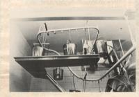
Dust and dirt problems are considerably reduced with this Bridgeveyor overhead conveyor, consisting of a steel plated, articulated chain running through a 1%-in.
